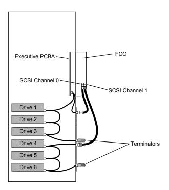
Figure 6-4 TLS-46xxx Cabling Diagram
